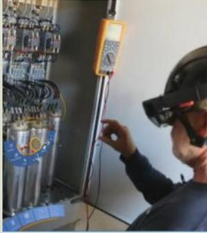
A Head Mounted Display (HMD) or tablet running MANIFEST enables an experienced field technician to easily “Author” an augmented reality content session using only voice and a few gestures (or keyboard for tablet). Manifest maps the actual equipment in 3D space using the HMD’s stereoscopic cameras. The technician places step-by-step instructions in 3D space around the equipment for others to utilize: job nuances permanently captured.
